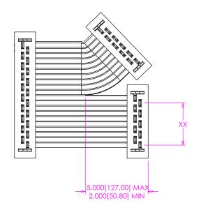
"XX" = NO. OF CONDUCTORS BROKEN OUT FROM THE FIRST POSITION.
